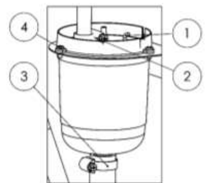
Fig. 6-4. Humidifier water level detector
